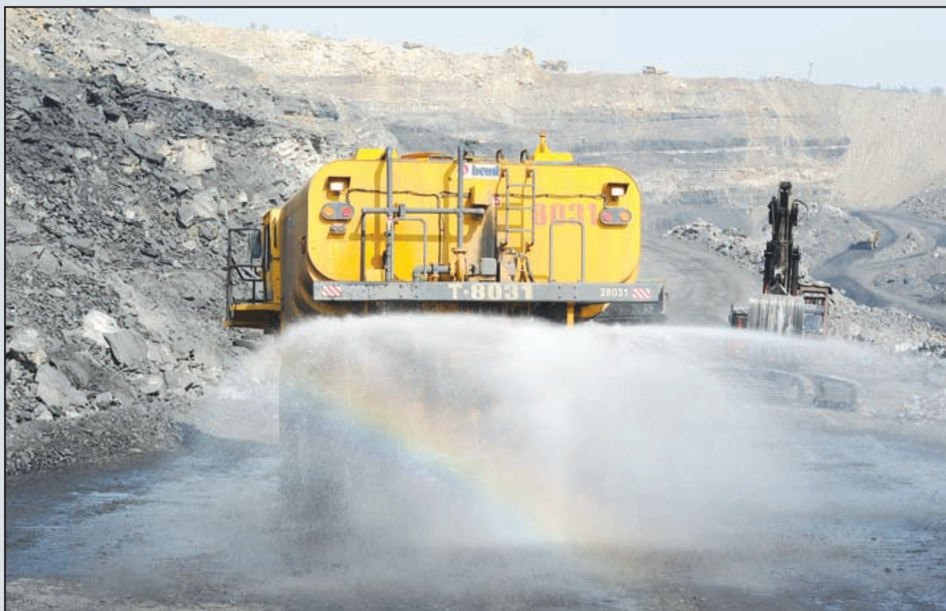
Eco-friendly activities are being practiced in Opencast mining - 35 KL Sprinkler spraying water on haul roads of Manuguru Opencast Mine
