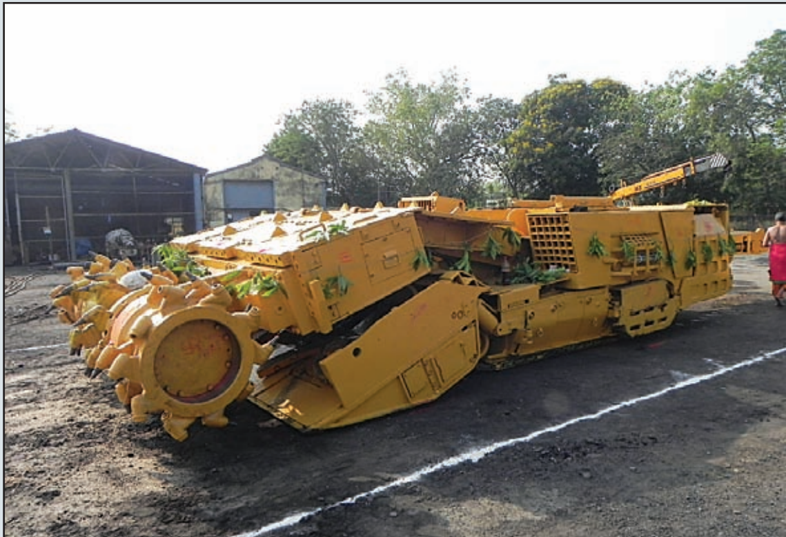
New Continuous Miner ready to deploy in underground mine at RG-I area
