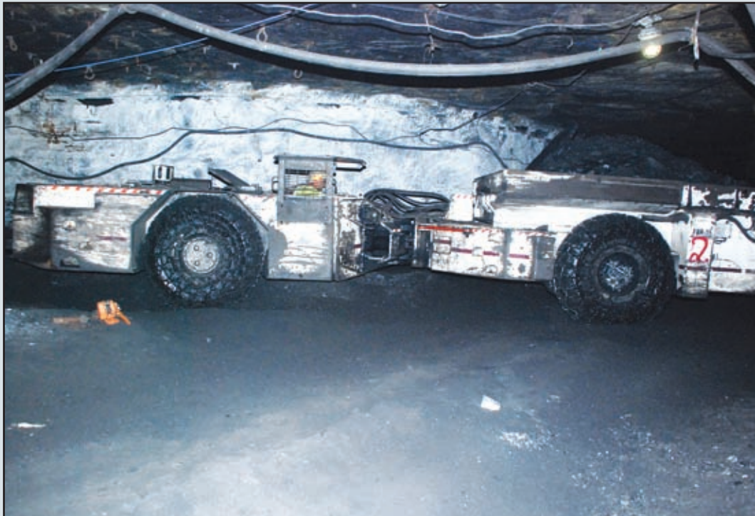
Load Haul Dumper at work in Kothagudem area mine
