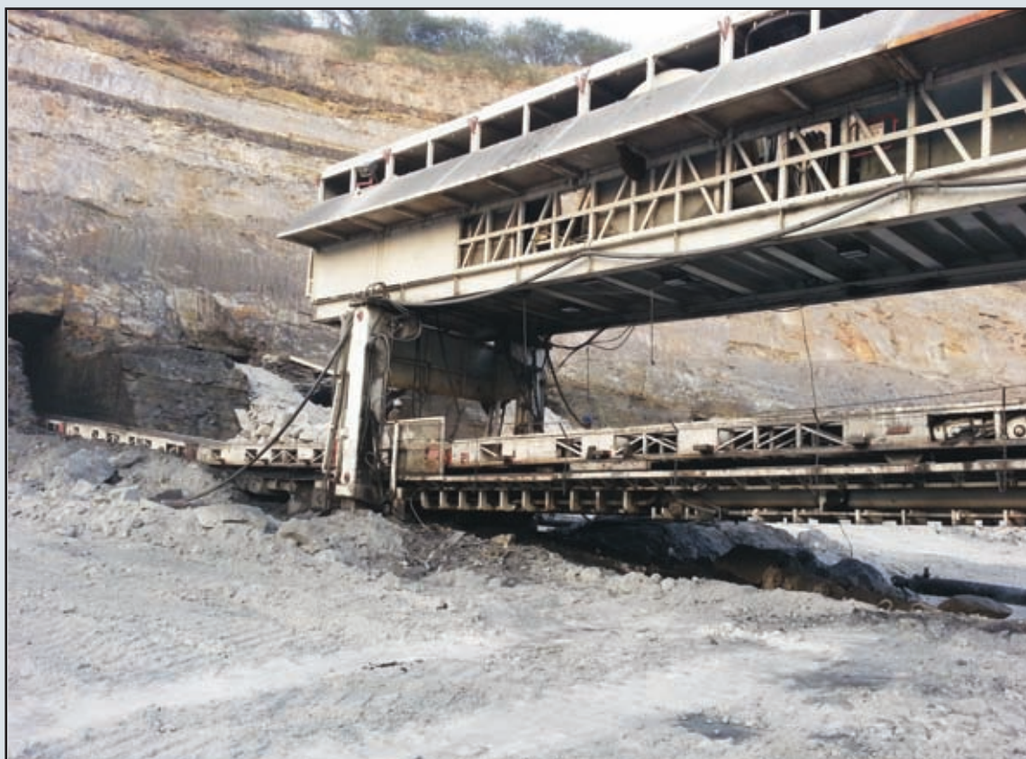
Production from Highwall mining technology at Medapalli Opencast Project, RG-I area
