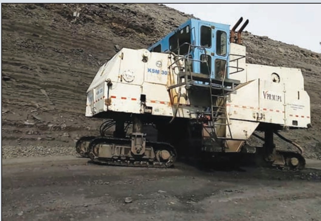
Production from Surface Miner technology at Koyagudem Opencast Project – Yellandu area
